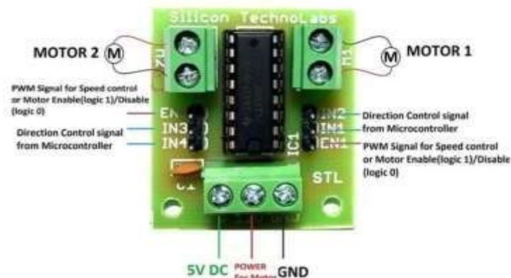
Fig 2: L293D Motor Driver
